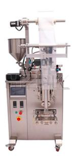
Automatic filling and sealing machine is suitable for all kinds of paste and liquid without gas, such as ketchup, sauce, oil and so on.
