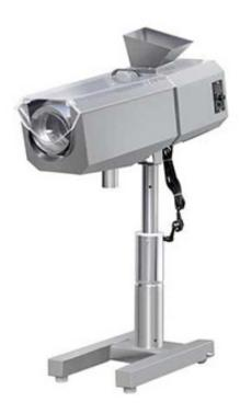
SPJ137 High Speed Tablet Deduster is an automatic continuous high speed tablet sifter, which can be attached to any type of rotary tablet press. Its function is to separate surplus powder absorbed on surface of tablets by the air vacuum suction, which accumulated during the pressing process. It also polishes the tablet edge by screen sifting and rotating.
