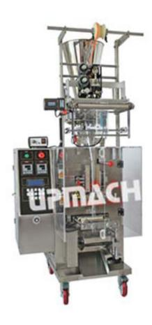
Granule Packing Machine is a vertical form fill seal machine that is used for sachet packaging of granular products, such as seasoning, monosodium glutamate, tea, sugar, coffee, pepper, desiccating agent and seeds etc. DXDK series sachet powder packing machines are widely used in pharmaceutical, chemical, foodstuff and other industries.
