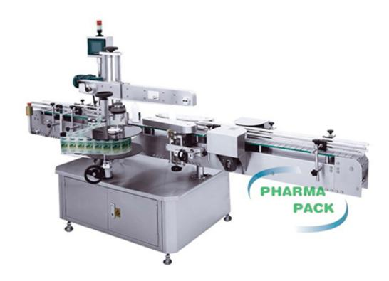
The bottle without label enters the rectifying bel t by bottle dis pen sin g wheel, two clamping belt orients bottle, and top belt keeps the bottle's pose. After the object detecting sensor senses bottle, it sends a dispensing label signal to la bel di spencer. At this time, bottle is labeled by label dispensing board. Meanwhile, the base paper is rolled back and label is labeled closely and levelly to bottle by the special device.
