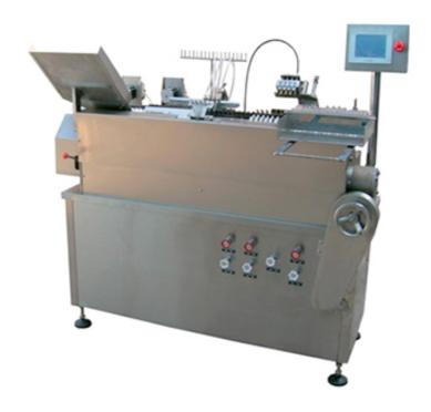
The machine is a new generation of the ampoule drawing, filling and sealing combined equipment for injections. It adopts the rectangular feeding instead of the traditional ampoule feeding methods. In such case, the feeding is steady with no easy broken ampoule. A modern clutch is mouthed under the ampoule feed hopper.
