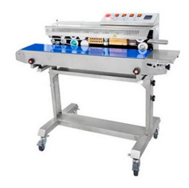
The machine can seal all kinds of heat sealable materials, which adopts constant temperature control system and stepless speed adjusting transmission mechanism.
