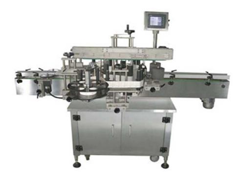
FBL-360 is economical, and easy to operate, equipped with HMI touch screen & PLC Control System. Built in microchip makes fast and easy adjustment and changeover. This automatic labeling system is ideal for flat and square container.
