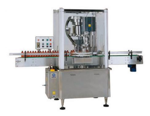
This machine is widely used for capping variety bottles in pharmaceutical, foodstuff etc industries.
