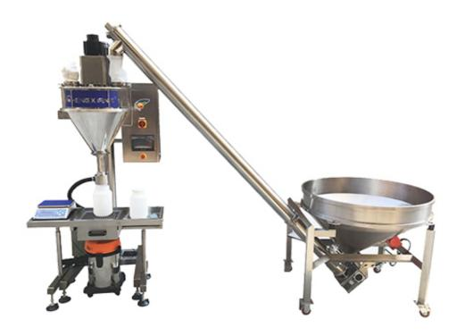
Semiautomatic filling packing machine is mainly composed of host, electrical distribution box filling of PLC, touch screen and electronic scale. The filling packing function complete measuring, filling, etc. The machine all stainless steel, corrosion resistance; PLC touch screen man-machine interface, display in both Chinese and English, the operation is convenient intuitive; Conform to and "GMP" certification
