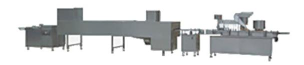
This cream production line is specially designed for filling, ultrasonic cleaning, high temperature sterilization drying, cooling, and sealing bottles with syrup, cream, cubilose, and many other liquids. Machines of this line can be used independently.
