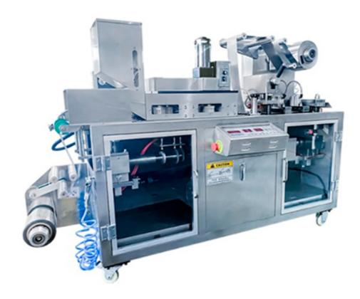
It is the latest product designed specially for middle and small sized pharmacy factory, preparation room of hospital, health care factory. It is adopted with micro-computer, touch panel operation, frequency speed regulation, adjustable stroke, convenience of operation, firm structure, well function; it is the ideal packaging equipment. It has passed Province technology production authentication.
