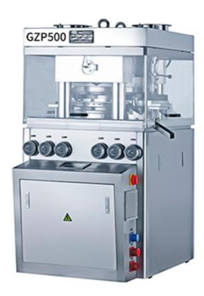
This machine is one kind of double side rotary tablet press machine, which can press granular materials into round shape tablet, irregular tablet or double-side engraved tablet.
