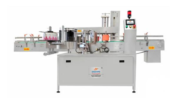
The Automatic Double-Side (Front & Back) Sticker Labelling Machine consists of the main structure, product in-feed screw, product transmission belt with guide adjustment, top product holding conveyor with height adjustment, 2 nos. of label dispensing unit, label pasting unit, motor, sensors, AC drives, motors, electrical panel, mains on/off, emergency switch, PLC & HMI.
