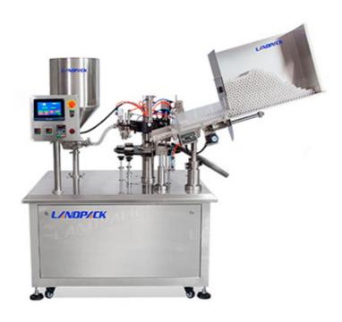
Commonly used in the filling and sealing of aluminum tubes, plastic tubes, and composite tubes in the cosmetics, paste, pharmaceutical, food, adhesive and other industries. It's the ideal equipment in cosmetics, pharmacy, food, and other industry.
