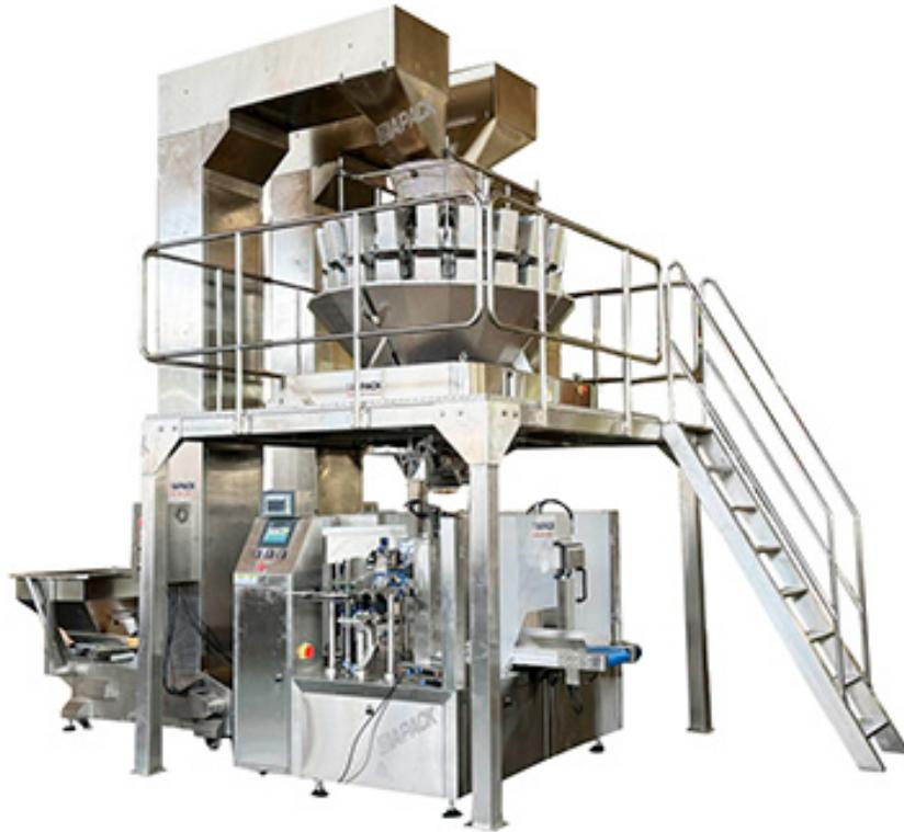
This unit machine including one set ZL20-1.6L multi heads weighing machine for weighing two different product, one set ZL8-230 rotary bag taking opening filling sealing machine, one set DT5 bucket elevator and one set safety platform and ladder. The main machine is control by siemens PLC and operate by touch screen. Adopt famous Electrical accessories. High automation and easy to operate. Widely use by the different industry like Daily chemical, food, chemical, and etc.
