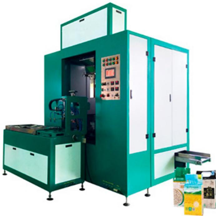
This machine consists of one set linear weigher for weighing and filling, one set bag given type vacuum packaging machine, one set take-off conveyor, it own functions of automatic weighing, filling, bag giving, vacuuming, sealing and taking off. It is suitable for granules, such as: rice, miscellaneous grains, beans, cashew nuts, etc.
