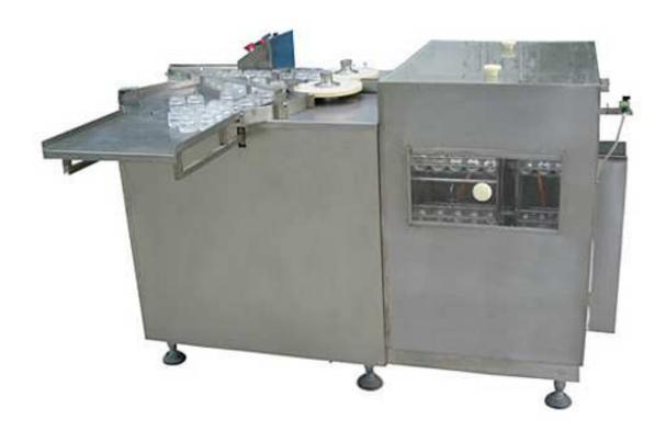
This machine is applied to clean the clinical bottle or oral liquid bottle with its revolving drum structure. Supply the bottle by feeding disk then transfer it through Wheel and input the bottle with revolving drum at interval. After passing through the ultrasonic water area, clean the bottle with recycling water (or tap water), distilled water and purified compressed air alternatively.
