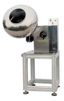
Tabletop machine for coated tablets is a subspecies of the pharmaceutical equipment which is represented by two models: TBY400 and TBY500.
