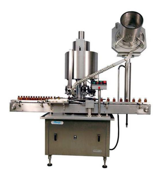
Automatic ROPP Cap Sealing Machine is versatile, self-supported on stainless steel leg with height adjustable adjustment system. The machine is precision built on sturdy welded steel frame completely enclose in stainless steel sheet and doors are providing to facilitate the servicing of machine.
