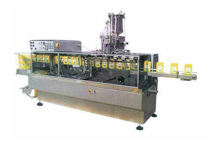
This type of machine is designed and manufactured conforming to European technical standards. This is an automatic machine, which has the integrated line of bag making, filling, sealing, and printing. The outside container materials are heat-sealing; finish packing of three-size, four-size sealing and stand-up bag by preparing various kinds of filling machines. It is the ideal machine in the industries from agricultural chemical, pharmaceutical, food, and cosmetics, etc.
