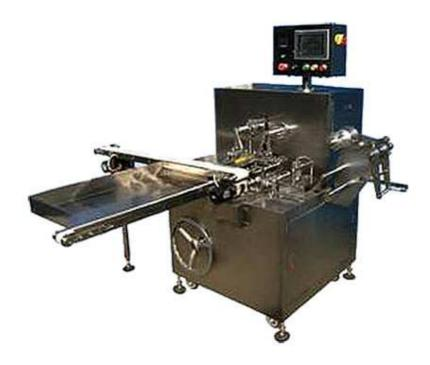
The DZB Type tablet packing machine is designed for the Tablet packing. It is the best equipment for packing the Chicken Flavor tablet, chocolate, sugar tablet. One machine could pack the tablet automatically. It is widely used in food industry.
