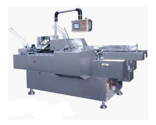
The machine is the high-tech products which integrates electricity, gas, light. The products is suitable for boxing or carton the Aluminum-Plastic blister card, medicine bottle, cosmetic, poker etc. The machine can automatically finish all jobs such as manual folding, paper box opening, and the stuff boxing or cartoning, bitch number printing, box sealing. It can be used alone or be linked with the other device.
