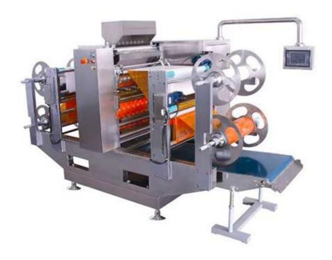
As shown in the picture, the multilayer pouch granule packing machine is used for packing loose, non sticky granule material in the medicine, food, daily chemical and other industries. It provides measuring and automatic packing into sachets such materials like Chinese medicine infusion, oatmeal, coffee etc. crystalline materials like monosodium glutamate, white sugar, salt etc. and small shot materials like Chinese patent drugs, dryers and so on.
