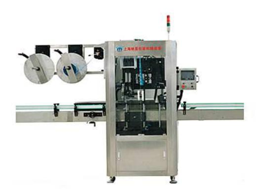
In order to meet the assorted demands of respectable clients, we are able to deliver automatic body shrink sleeve applicator. The offered range of automatic body shrink sleeve applicators is designed & developed utilizing optimum grade material, sourced from trusted vendors of the market. Along with this, the offered range of automatic body shrink sleeve applicators is strictly checked on myriad parameters to ensure its adherence with the benchmarks of quality.
