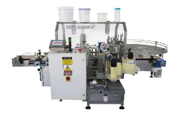
SA's CAROLUS series is the first labeling system developed specifically for buckets that includes a proprietary precision orientation system – which ensures that the label is placed in exactly the same position on each and every bucket.
