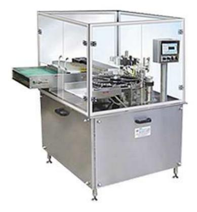
Suitable for wrap around labeling on Ampoules / Tubular vials or any other thin dia. Conveyorised tray loading and tray Collection system Spot wrap around system for accurate labeling. Star wheel with spring loaded rollers to take care the variation in dia. in case of 400 speed model. Available with latest Digital SERVO technology to achieve higher speed.
