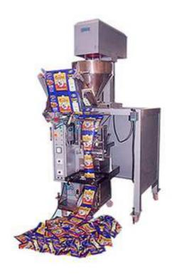
Auger base ffs machine is one of our form fill seal machines which are manufactured with high degree of precision to handle diverse type of non free flowing powdered products (Also known as powder packing machine) like Custard Powder filling and packing, Roasted Ground Coffee, Spices, Talcum Powder packaging, Detergent Powder packing, Pharmaceutical Powders, Dyes and Coloring agents Powder, Distemper Powder, Pesticides etc.
