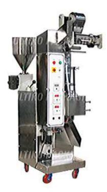
The MK-103 is an small automatic vertical form fill seal packaging (VFFS) machine designed to package pastes, semi-viscous and viscous products. This machine uses volumetric paste pump dosing system and is integrated with continuous type sealing system to produce 3 side sealed and 4 side sealed pouches / bags.
