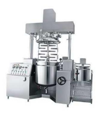
Vacuum emulsifying homo mixer is widely used in Skin care cosmetic, pharmaceutical and food industrial. We offer different type of these machines, such as top homogenizer, bottom homogenizer, single hydraulic lifting, double hydraulic lifting, button control and PLC control for our customer's selection.
