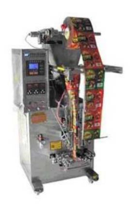
This machine is widely applied for food, pharmaceutical, and chemical products in mesh size range from 120 to 400, such as milk powder, soya powder, cosmetic powder, slimming tea, medical powder, etc.
