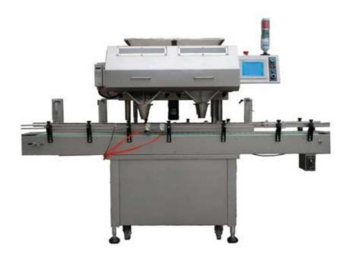
The high-speed tablet & capsule counting and bottling machine adopt 24-channels. Compact design with dual-track conveyor can enhance the capacity of output. The GS-24 is equipped with advanced LED sensor which can count and fill all standard and irregular shapes and all sizes of tablet, capsules, caplets, pills with 100% accuracy.
