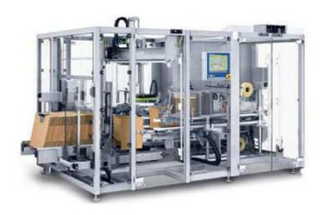
Includes automatic machines for the packaging of pvc bottle, pet bottle, glass bottle, paper and box in corrugated cardboard cases and/or trays without film which widely used in food, toy, chemical, cosmetic, medical and plastic industries. Wrap around case packers can achieve an output up to 35 packs per minute, according to the product. The packing arrangement can vary according to the containers shape and dimensions; in general, the most requested arrangement are: 2x3, 3x4 and 4x6.
