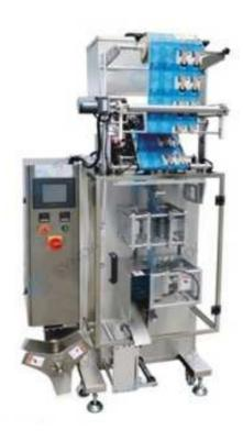
K150B-R Automatic Sachet Vertical Packing Machine is specially designed for small particle products automatic weighing & bag form fill seal at high speed. This machine unit adopt back rushed round style for small sachet packaging.
