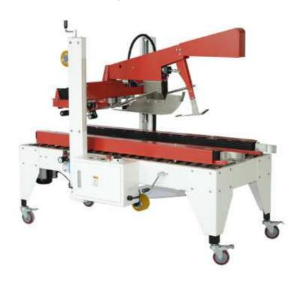
This machine's quality is better than so many carton sealing machines in Turkey. It is designed for saving time, and working with less worker. This machine takes undone carton, close its flaps and seal the top and bottom.
