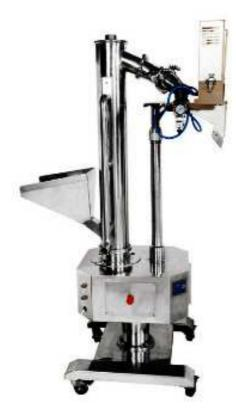
The machine has the multi-function of polishing, lifting and sorting capsules. Entrance of the machine can be connected to various types of capsule Filing machine's outlet. Its outlet can also be connected with metal detector. Realization an even machine production mode of polishing, lifting, sorting, testing and monitoring.
