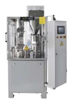
NJP-800C automatic capsule filler processes the products for optimal productivity up to 800 capsules per minutes, featuring low-maintenance operation, minimal downtime, and overall dependable production.
