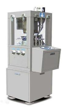
The ZPS8 rotary tablet press is a small intelligent machine that is applicable for making tablets of small batch in drug research and development center in pharmaceuticals industry, laboratory, etc.
