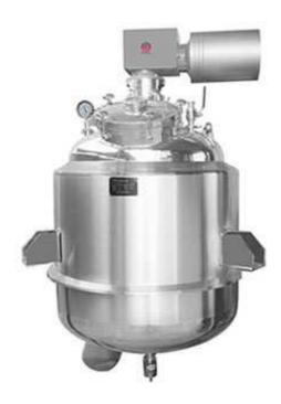
The medicine mixing tanks are designed and manufactured based on the medicine preparation process or client's specific requirement. The specific three-layers structure, inner layer, jacket and insulation layer, is applied to ensure a even heating and working efficient. Not only it can been used in pharmaceuticals industry, but also in cosmetics industry, food industry, liquid industry can been found it's application.
