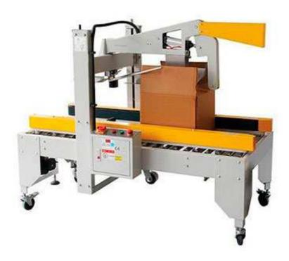
The machine is suitable for paper carton erecting automatically. It has function of cover-folding, sealing bottom with tape. It is economical and it is with high high-efficiency. It is ideal automatic carton forming and bottom sealing equipment.
