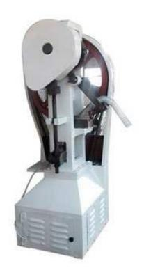
This machine is a medium flower basket type tablet press machine, applicable to the pharmaceutical, chemical, food, electronics, fuel and other industrial sectors. Is to deal with all kinds of granular raw materials into tablets agent basic equipment.
