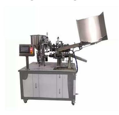
Mainly used for packaging materials with aluminum tubes. This machine is widely used in packaging in the pharmaceutical, daily chemical, food, chemical and other industries. Such as ointment, toothpaste, epoxy glue, 502 glue, hair dye, and other liquid or paste-like materials filling and sealing.
