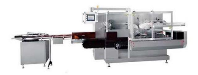
This machine is used to take Alu/PVC medical plate or plastic bottle (vitreous bottle) to filling in paper box automatically. It can perform automatically the whole process of folding and conveying of leaflet, paper box forming, batch number printing and box sealing. The machine can also be linked to work with Alu/PVC packing machine, bottle filling machine and transparent film three dimensional packing machine.
