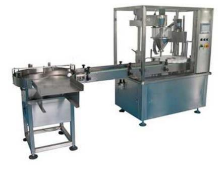
The monobloc machine can finishing measuring, filling capping etc. because of original design, it is more suitable for packing powdered material that is easy to flow, like veterinary drug, sugar, glucose, carbon dust, talcum powder, essence etc.
