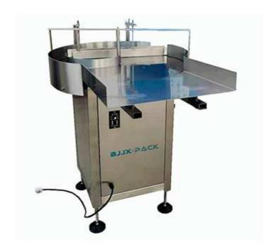
Put the bottles (plastic bottles, glass bottles) on the rotating disc manually, and then it will set the bottles into conveyor in orderly.
