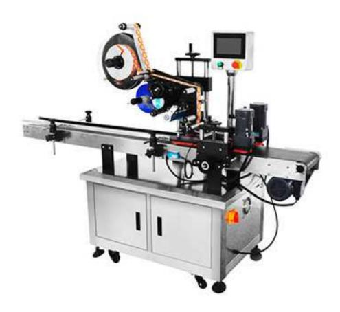
This is a high-speed flat labeling machine that can quickly label perfume bottles, shower gel bottles and other flat bottles.
