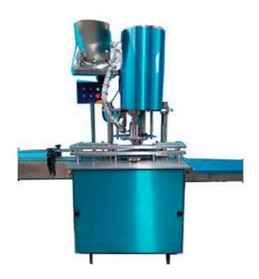
Automatic capping machine can respectively press pattern and close over for aluminum cap and seal plastic rotary cap, other compressing plastic cap and iron cap of triangle feet. Working head is made according to sample of bottle and cap user provides. The product is designed in first rate, structure is reasonable, appearance is beautiful, adjustment is convenient, practicability is strong and product is deeply praised by users depending on first quality.
