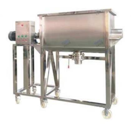
This is a ribbon blender, designed to mix all kinds of dry powder. It consists of one U-shaped horizontal mixing tank and two groups of mixing ribbon: outer ribbon displace the powder from the end to the center and inner ribbon move the powder from the center to the ends. This is the principle of ribbon blender working principle.
