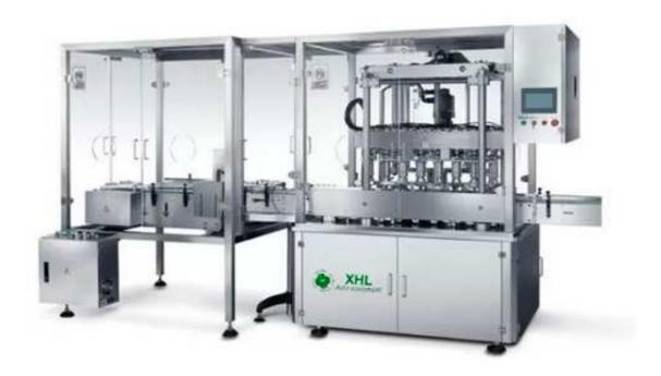
The series of products are mainly used for aseptic filling of serum, cell culture medium, etc. in such industries as medicine, biology, etc. The production line inherits internationally advanced technology in its structural principle, and incorporates various patented technologies with independent intellectual property rights. It has reached the advanced level and can replace similar imported products.
