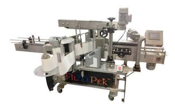
The Automatic Vertical Sticker Labelling Machine is one of the most users friendly. The machine is used for full/partial labeling on different size of flat or rectangular containers. The automatic model is equipped with roller spacing device resulting in a simple operation with "No change parts required".
