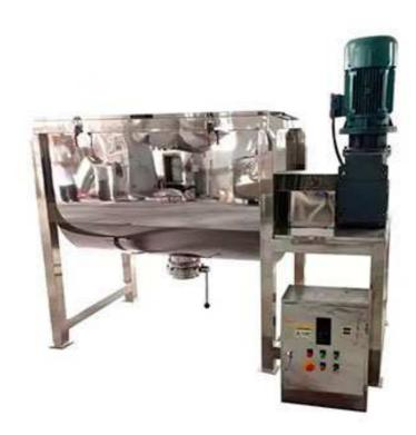
Double screw ribbon Blending Machine Industrial Blender for powder is a mixing equipment with high efficiency, high uniformity, high loading coefficient but low energy cost, low pollution and low crush. The special design of double ribbon mix the materials into high uniformity in a few minutes. The Mixer Machine suitable for mixing a wide range of materials such as powder-powder, power-liquid, especially for paste, thick materials.
